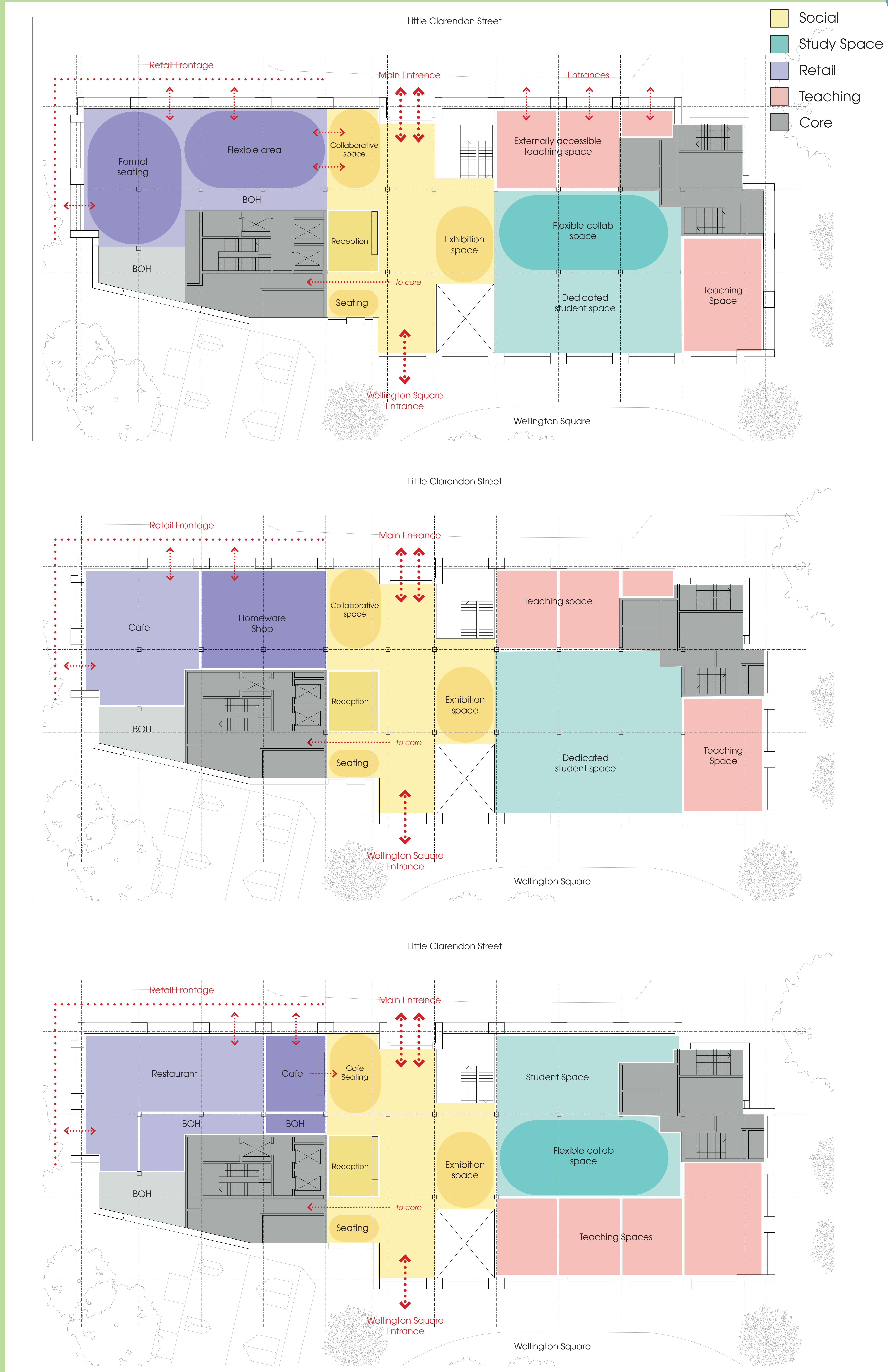
Indicative layouts showing flexibility of the ground floor of the new 25 Wellington Square
