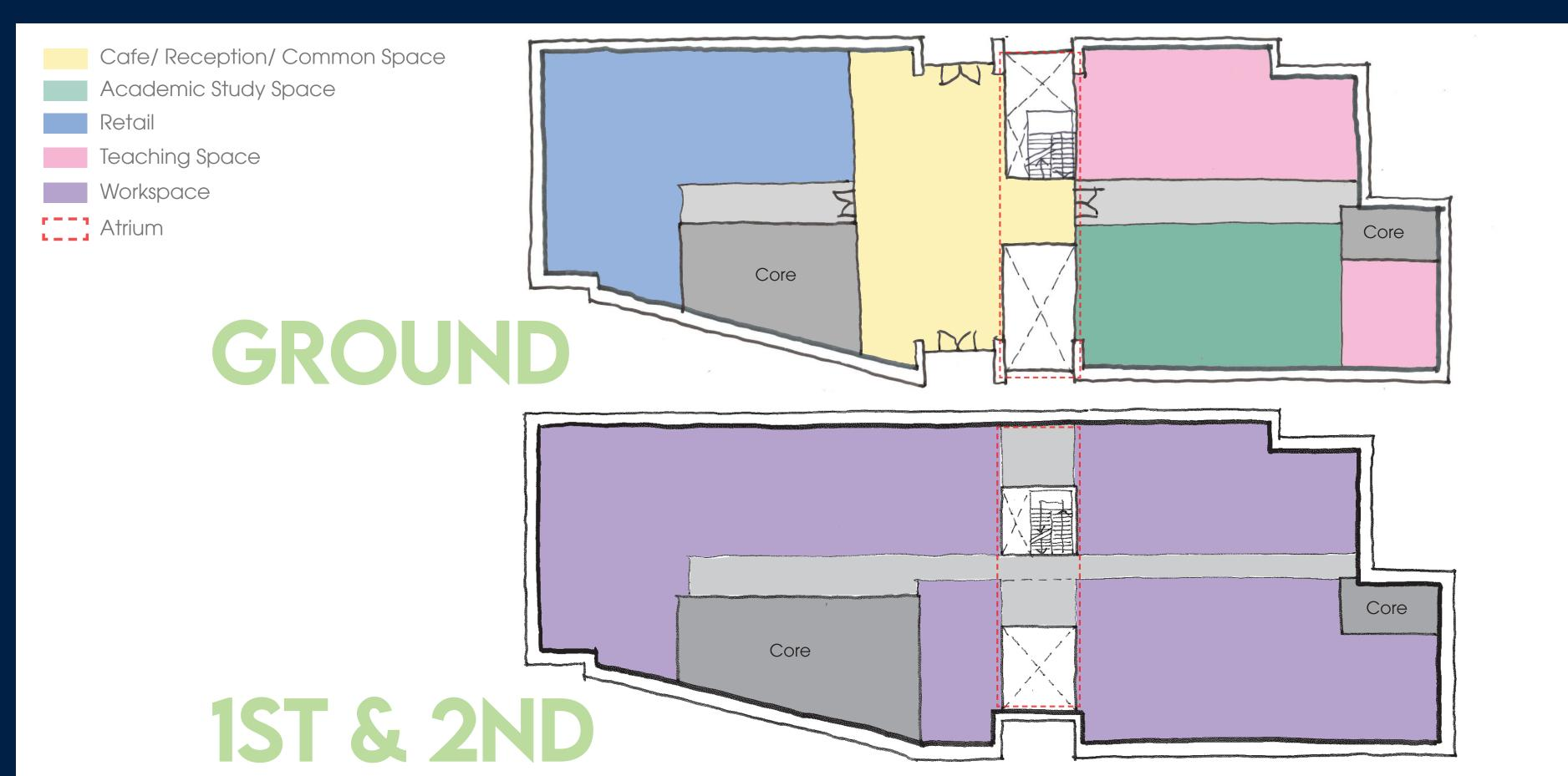
Internal plans of uses for ground, first & second floors
