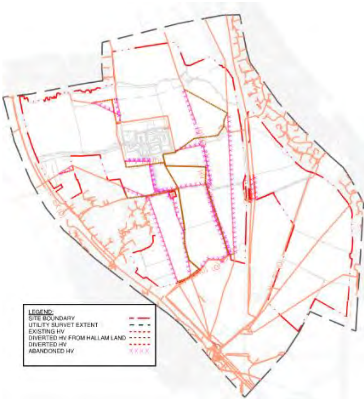
Figure 5—1 Proposed Electrical Diversion Routes
