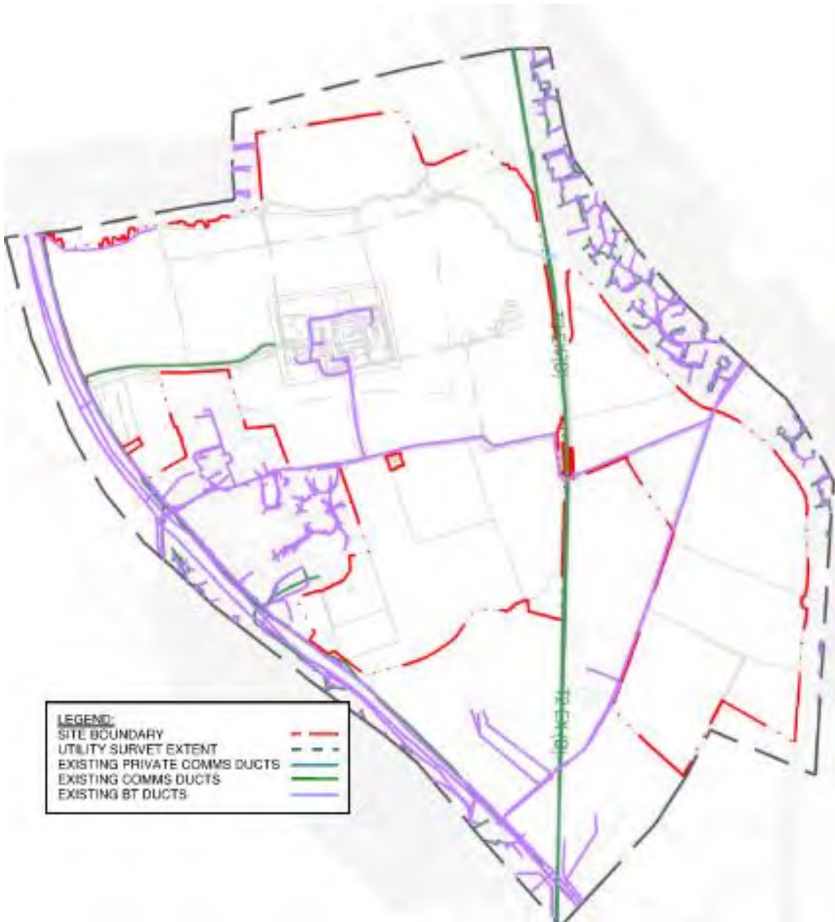
Figure 3—4 Existing Openreach Network
