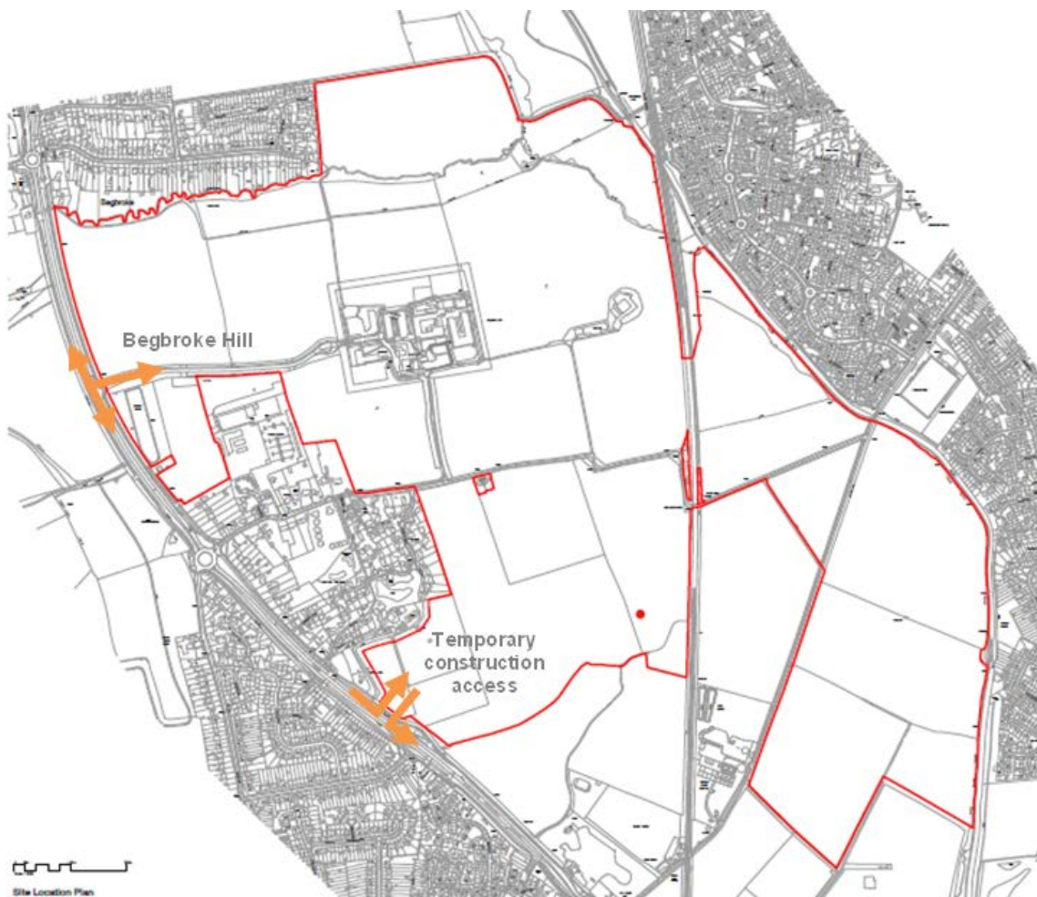
Figure 9.5: Proposed Construction Access Arrangements
