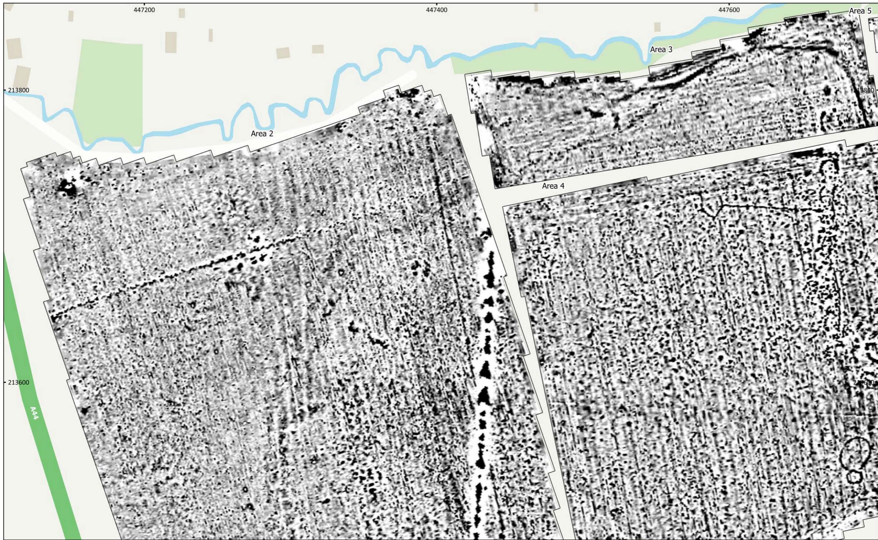
MSSP1306 - Begbroke, Oxfordshire Figure 29 - Magnetic Gradient (Areas 2, 3 & 4) 1:1,500 @ A3 Copyright Magnitude Surveys Ltd 2022 Contains Ordnance Survey data © Crown Copyright and database right 2022
