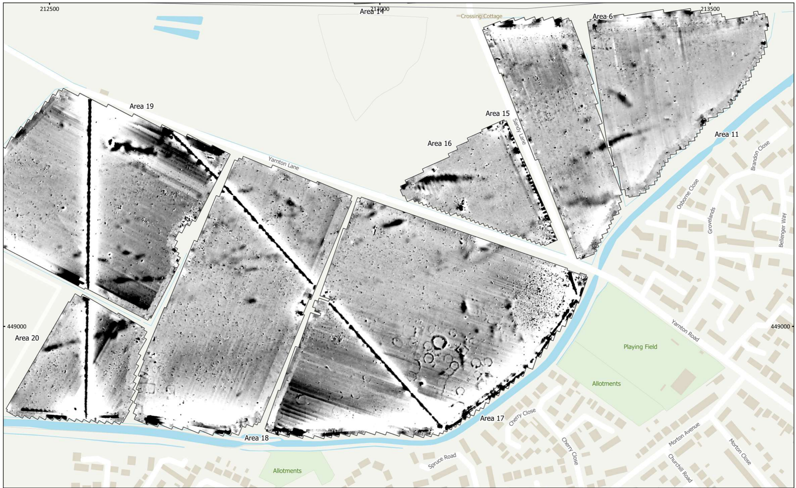
MSSP1306 - Begbroke, Oxfordshire Figure 21 - Magnetic Total Field (Lower Sensor) (Overview) (East Area) 1:3,000 @ A3 Copyright Magnitude Surveys Ltd 2022 Contains Ordnance Survey data © Crown Copyright and database right 2022
