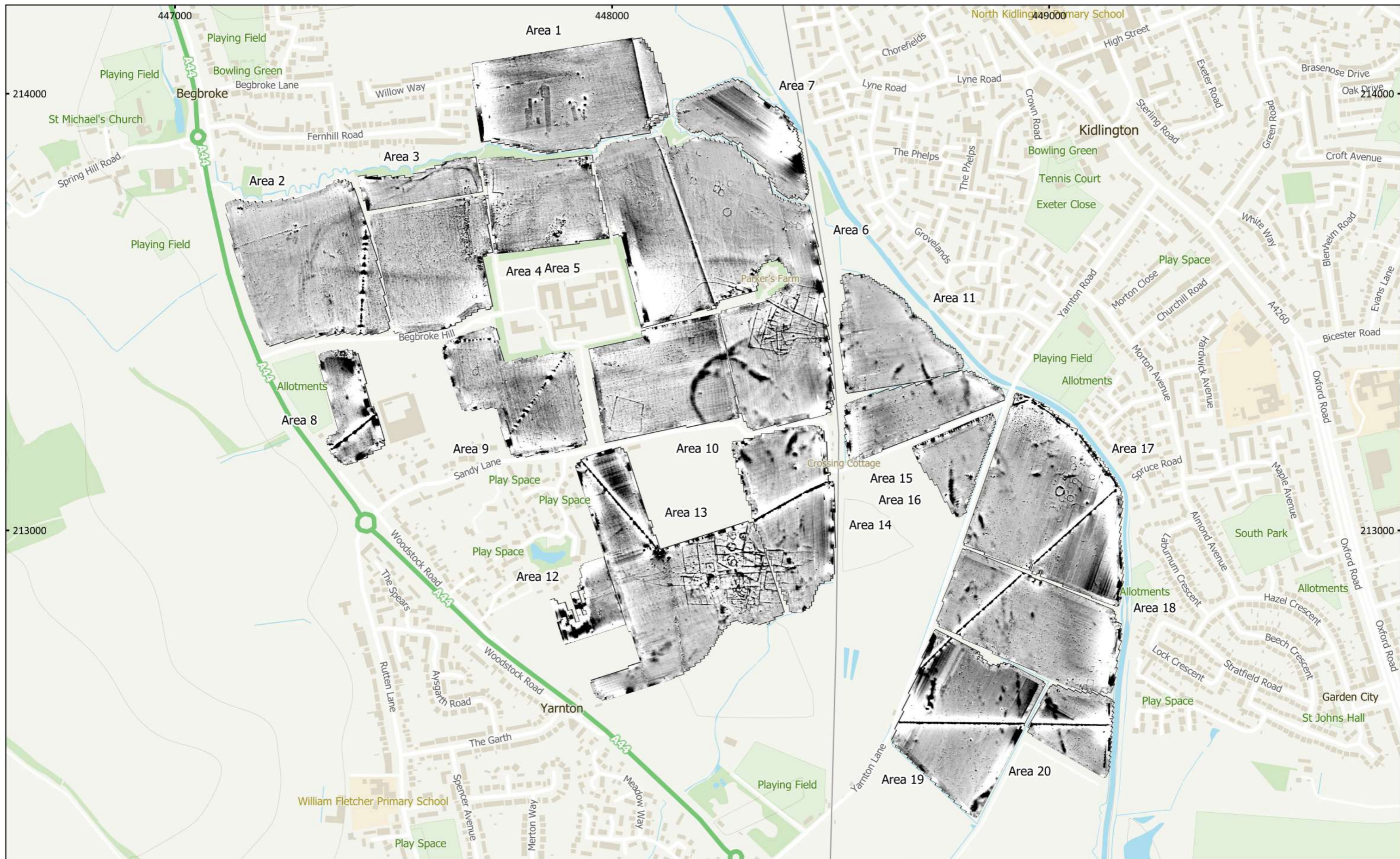
MSSP1306 - Begbroke, Oxfordshire Figure 10 - Magnetic Total Field (Lower Sensor) 1:8,000 @ A3 Copyright Magnitude Surveys Ltd 2022 Contains satellite imagery © 2022 Bing Satellite
