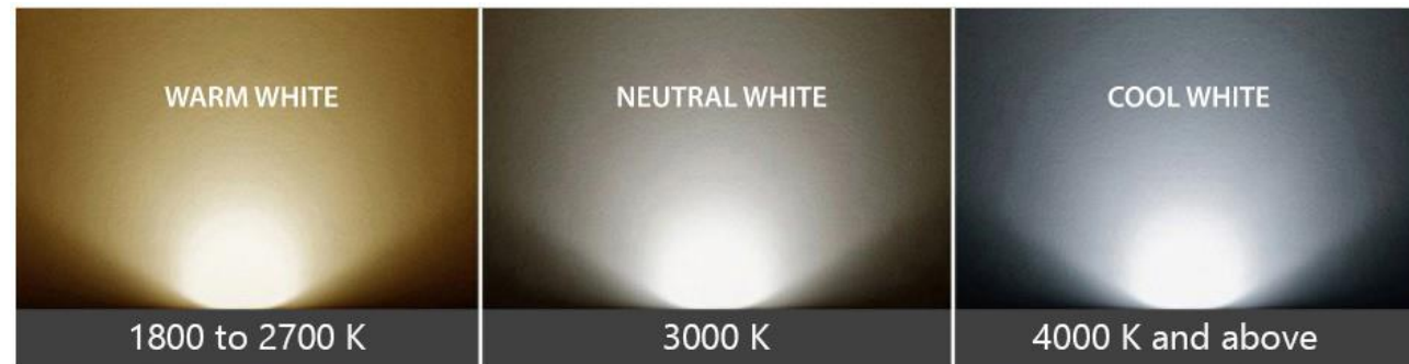
Figure 5.3 - Light colour temperature example chart
