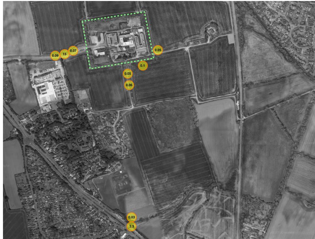
Figure 2.16 – Existing Illumination levels outside of Begbroke science park noted in values of Lux.
