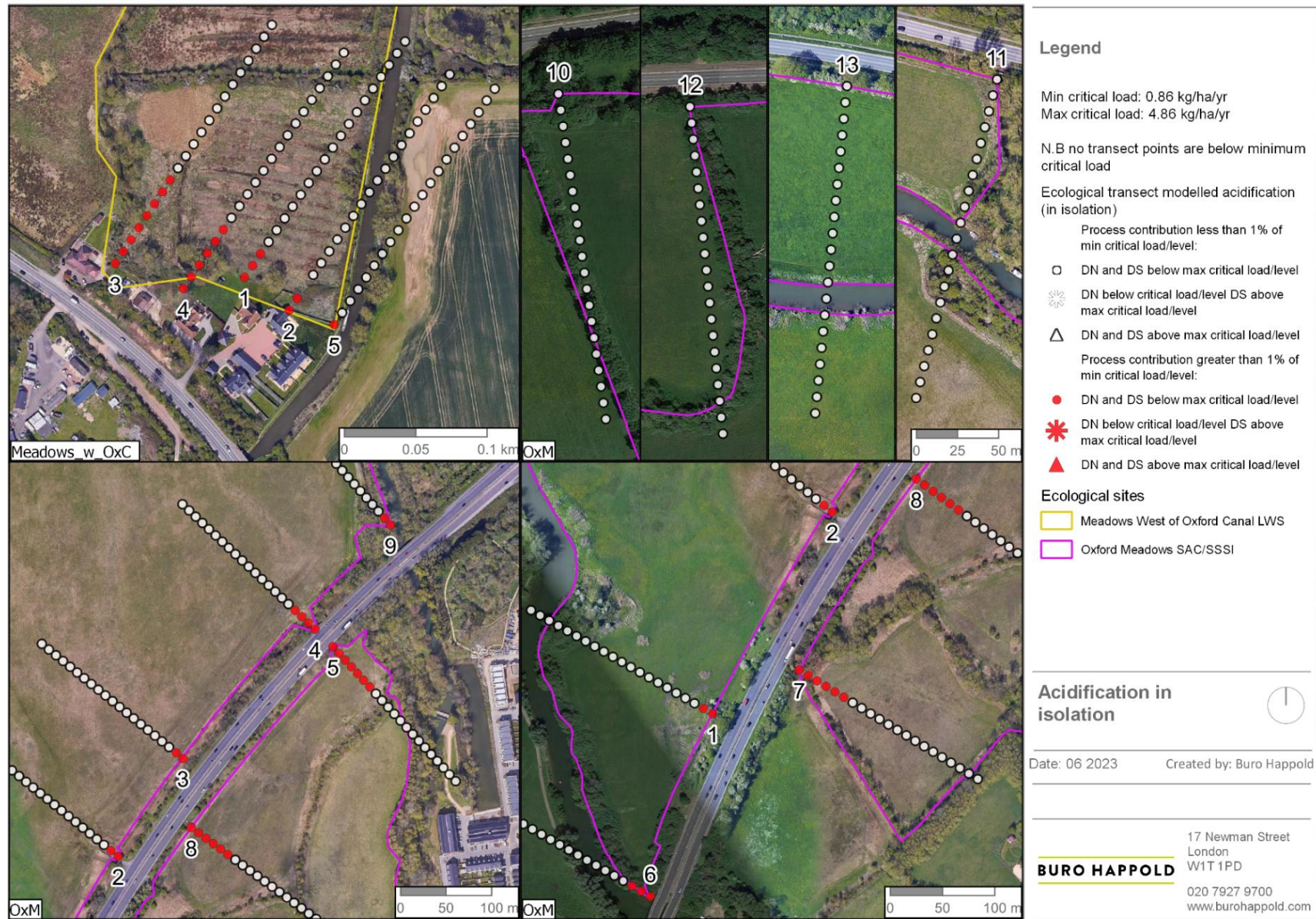
Figure 1 Modelled transect results - acidification in isolation (Oxford Meadows SAC and Meadows West of Oxford Canal)
