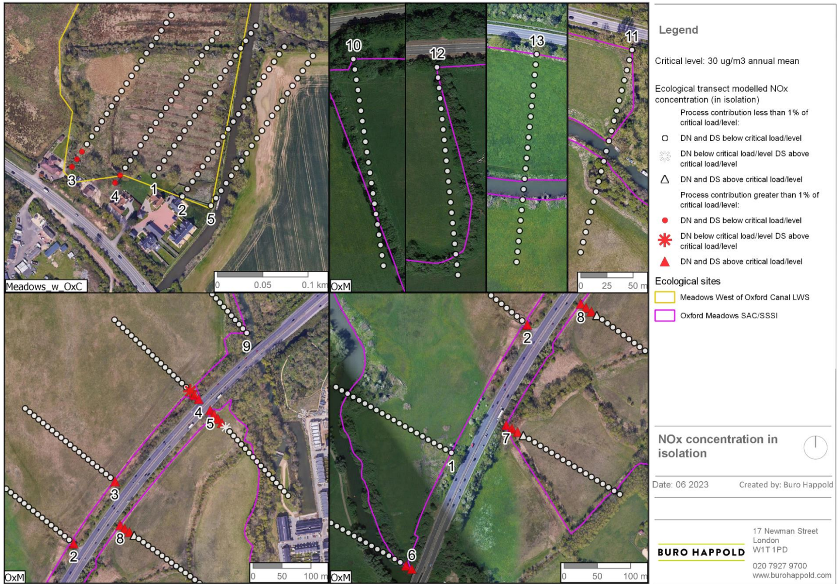
Figure 13 Modelled transect results - NOx concentration in isolation (Oxford Meadows SAC and Meadows West of Oxford Canal)
