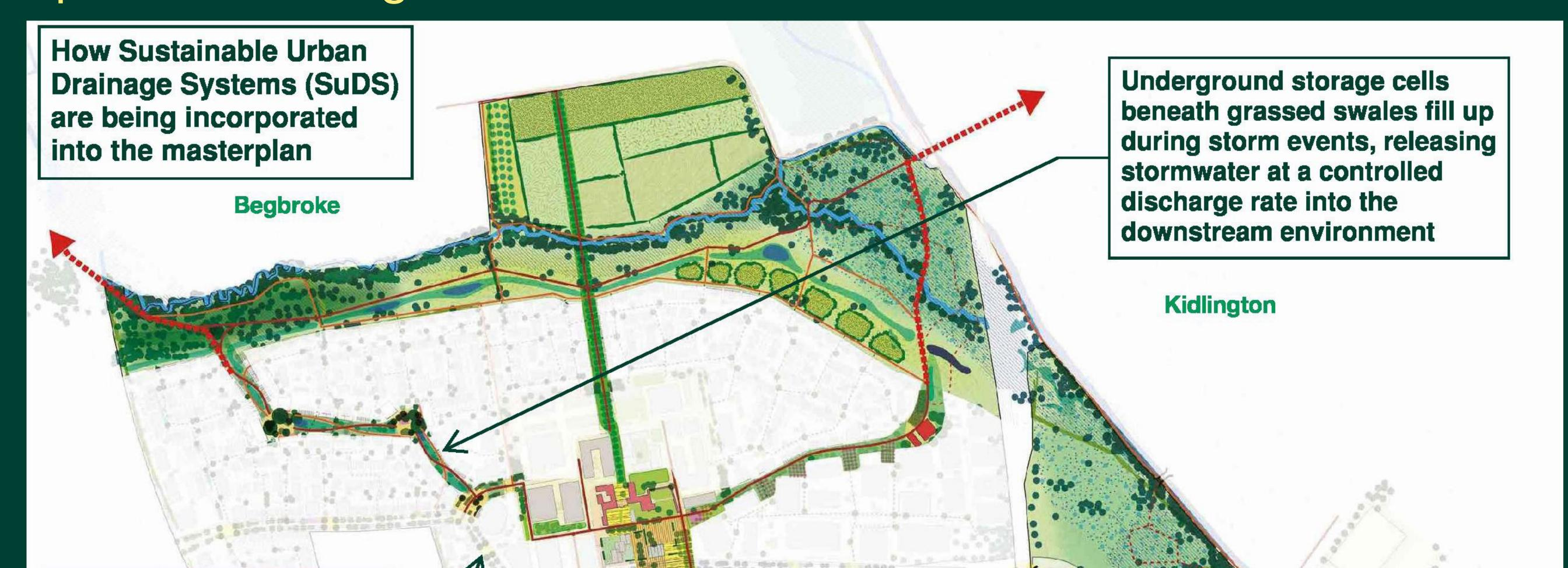
Grassed conveyance channels (swales) along roadsides pick up and treat stormwater runoff from roads
